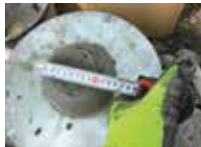
Measuring flow spread
