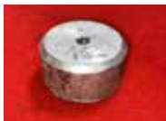
Adhesive strength test die
