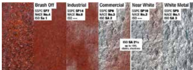
Standard degrees of cleaning for steel reinforcement
