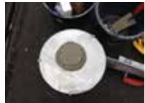
Flow spread measured on a Hagermann table
