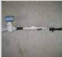
Injection lance with lamella drive-in packer (right)
