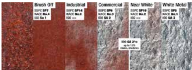
Standard degrees of purity for steel reinforcement
