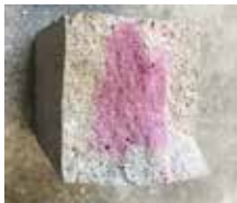
Testing depth of carbonation
