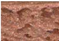
Substrate after blasting
