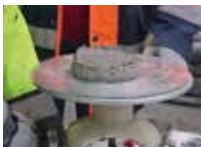
Measuring flow spread
